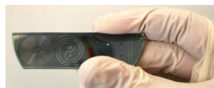
Microfluidic chip for determining supercritical conditions (P, T).
